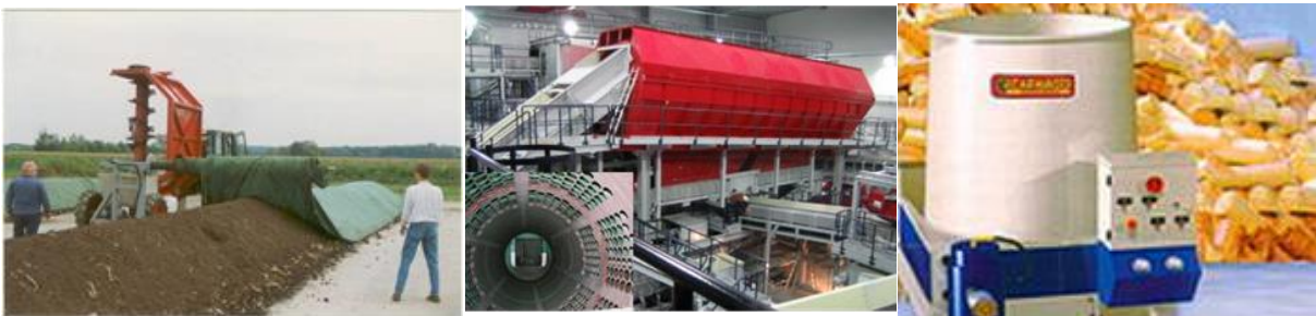
Figure 6. Principle of field composting, Beccari static chamber for composting and briquetting machine [6]
