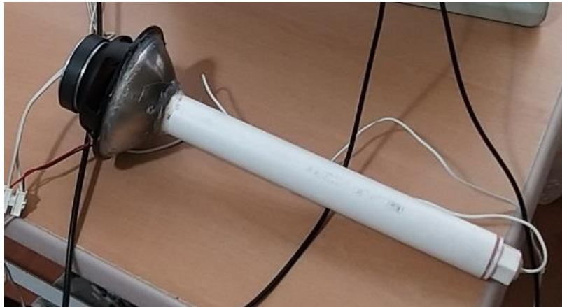
Figure 4. The combination of the resonance tube and the speaker with the conical part.
