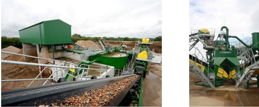
Figure 5. Complete recycling line composed of CDE Global machines
