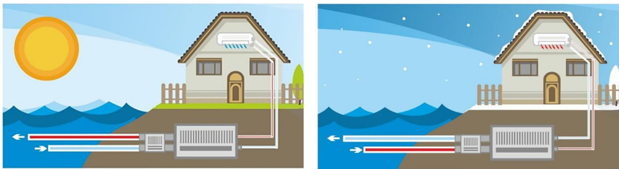
Figure 5: Sea water heat pumps– water in the mode of a) cooling; b) heating
