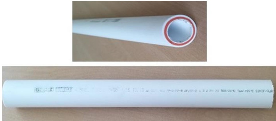
Figure 3. PVC pipe used as resonance tube.
