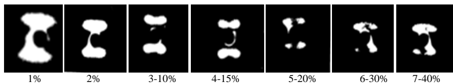
Figure 4. Small-angle radiographs of LDPE oriented at room temperature (1) then free-shrunk at T=100\text{ }^{\circ}\text{C} (2), re-stretched at room temperature (3)-(7)
