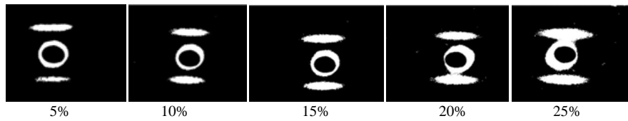
Figure 3. Small angle radiographs of high-pressure polyethylene (LDPE) stretched at room temperature after orientation at T=1000\text{ }^{\circ}\text{C}
